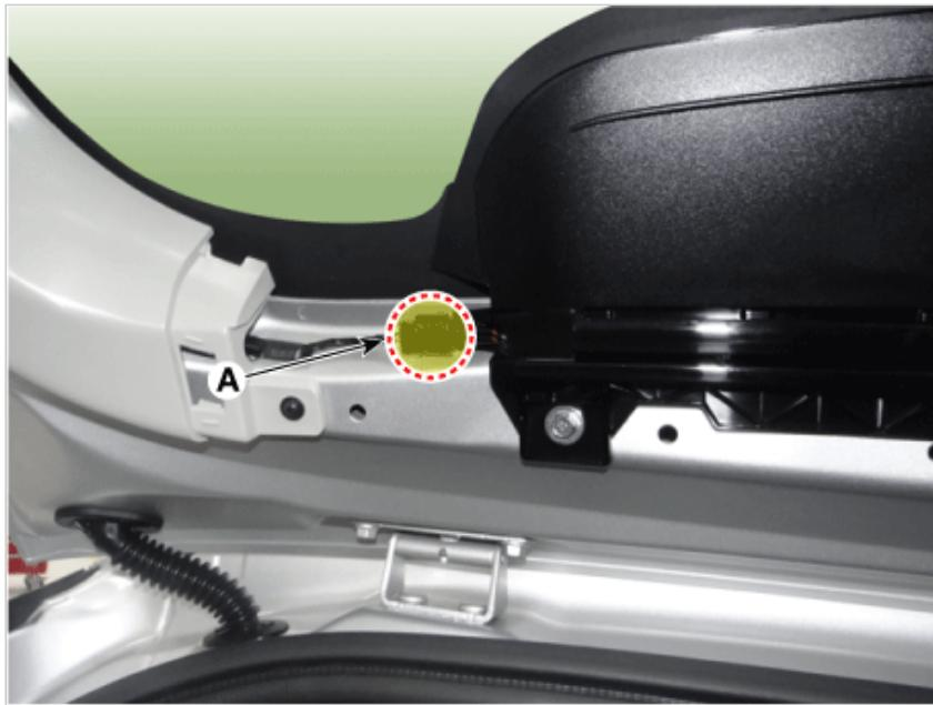
8. Remove the high mounted stop lamp (A) after loosening the mounting bolts.
