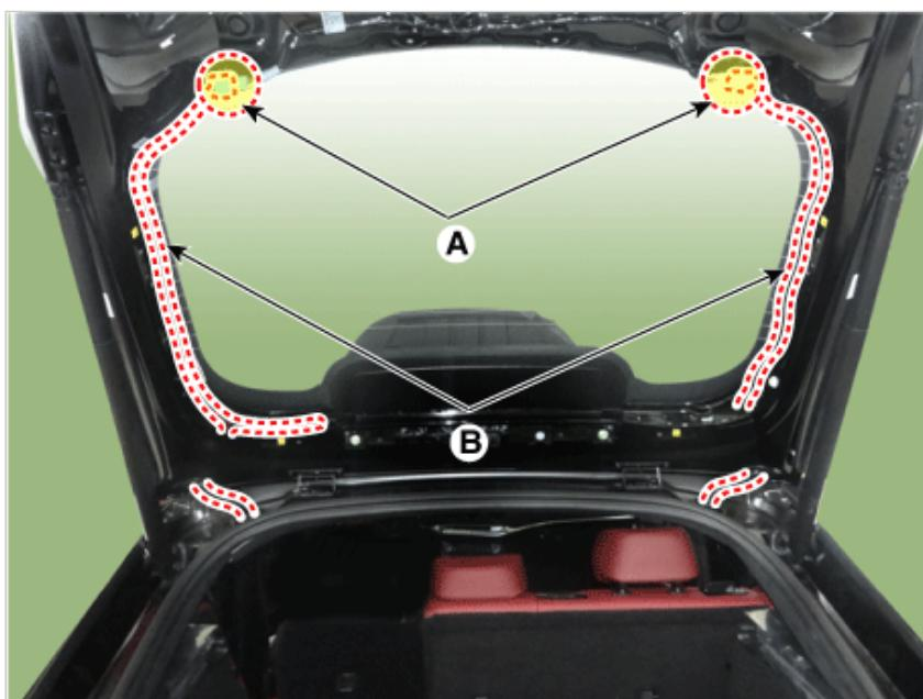
10. Using a screwdriver, separate the both ends of the tailgate lifter (B) after removing the socket clips (A).
